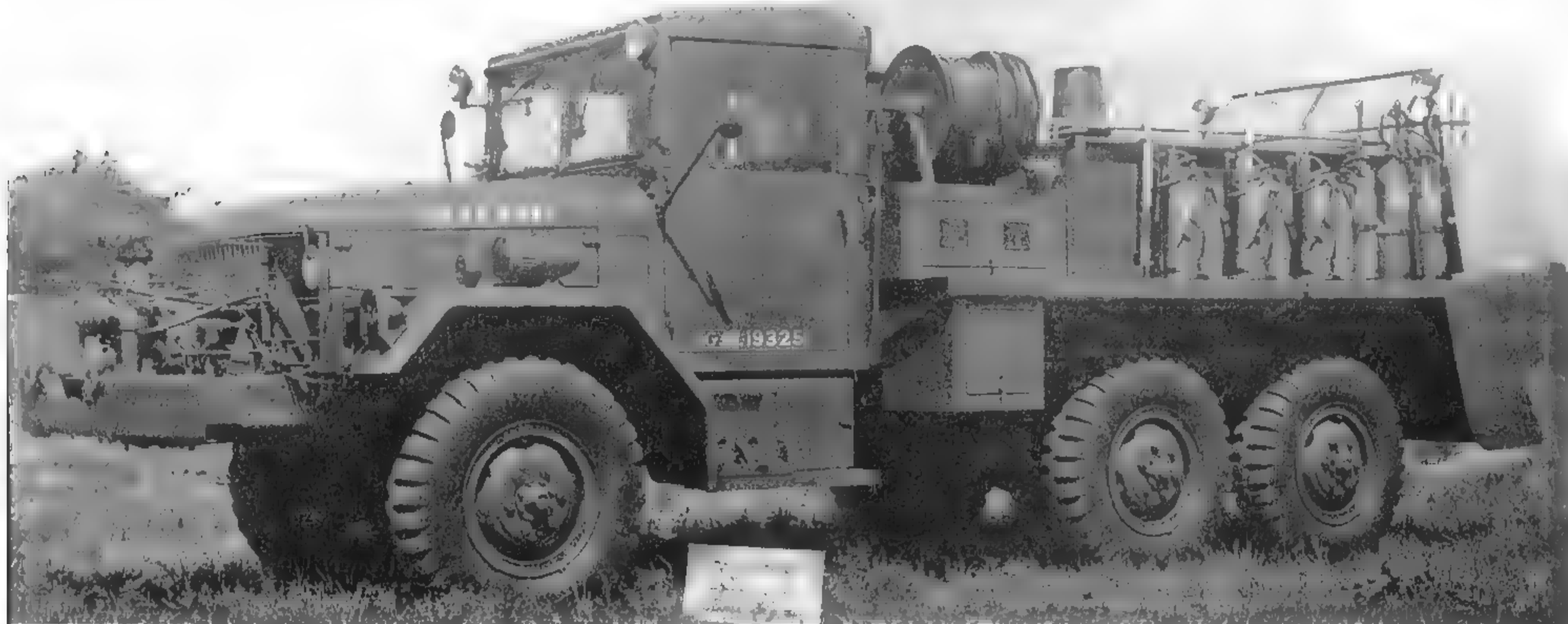
The 530A trucks were the first series of fire trucks built on the G-742 chassis. This Howe builder's photo shows the front-mounted pump and exposed equipment stowage characteristic of this series. (Photo courtesy of Richard Adelman collection)
